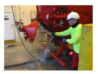
E78 Cleaning with high pressure water of fill- and discharge opening lids, rims included, lids and all joined parts
